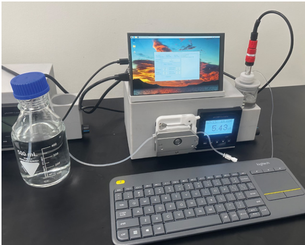
澳大團隊開發的「厭氧發酵」監測系統 The automatic analyser for volatile fatty acid (VFA) and alkalinity developed by UM researchers
