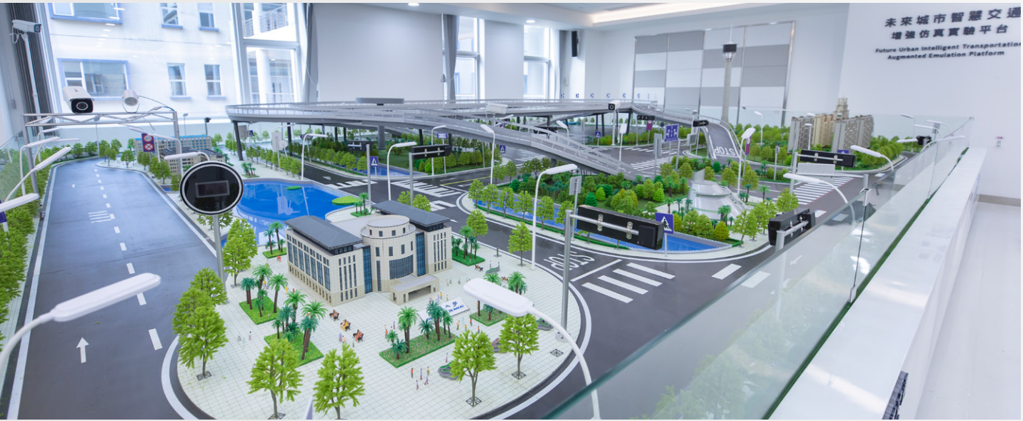
研究人員可在設於智慧城市物聯網國家重點實驗室(澳門大學)的實驗平台用模型車輛測試自動駕駛技術 This testbed in the State Key Laboratory of Internet of Things for Smart City (University of Macau) allows researchers to test their self-driving strategies on mini-cars in a mock urban scenario
