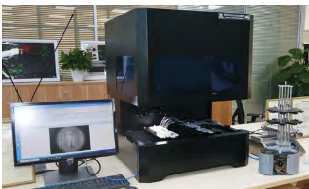
基於微流控技術的斑馬魚篩選系統 A zebrafish screening system based on microfluidic technology
