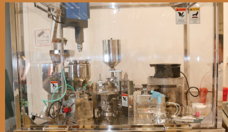
澳大自主研發的多態一體化膠囊填充機 The multi-phase capsule filling machine developed by UM
