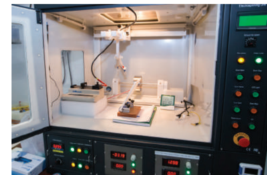
生產杜仲敷料的儀器 The equipment used to make EU-based wound dressings
