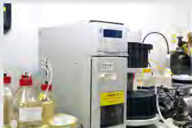
液相色譜質譜聯用儀(LC-MS)是創院時購買的首批啟動儀器，這些先進儀器為學生創造了多篇享譽國際的SCI論文。 Liquid chromatograph-mass spectrometers are the first batch of devices purchased by ICMS after its founding. These advanced devices have helped students to produce numerous internationally-recognized SCI papers.
